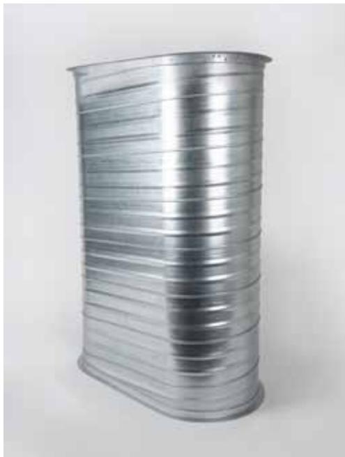
Oval ducts have very similar characteristics and advantages, as spiral rounded ducts. They are made from spiral tubes by hydraulic stretching. The features of the flat oval duct make it a very good option for designers and HVAC designers when the space limitations do not allow the use of round and rectangular ducts. The rounded corners do not create turbulence inherent on the rectangular air duct. This allows for higher volume and speed transmission without generating noise and dynamic losses.
