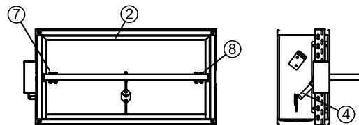
• The activating element - the specially incorporated fusible plate (8) reacts if the temperature the air passing through the valve opening exceeds 65 ° C. When this temperature is exceeded the solder melts, the closing spring mechanism (3) activates and closes the movable fire panel (2). The opening (7) is to perform a status review of the activating element (8) and, if necessary, for its replacement.
