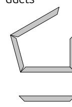
The sum total of 3 sides of the duct is equal or below 1080 mm.
