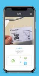
Connectivity card. The card will report a unique Activation ID (QR code) identifying the license for a specific Small Inverter Chiller unit controller. The Small Inverter Chiller controller has a sticker that must be sticked on the Connectivity card in order to use it with the app.
