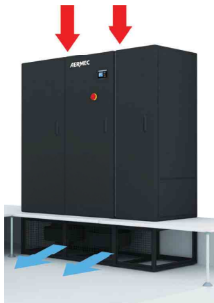
Standard execution for perimeter installation inside Data Centres: the height of the raised flooring must be minimum 550 mm.
