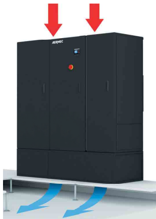
Execution for perimeter installation inside Data Centre. In this case, the sub-base side closure panels must be installed above the flooring. It is in any case essential to make sure that the height of the ceiling allows good air intake.
